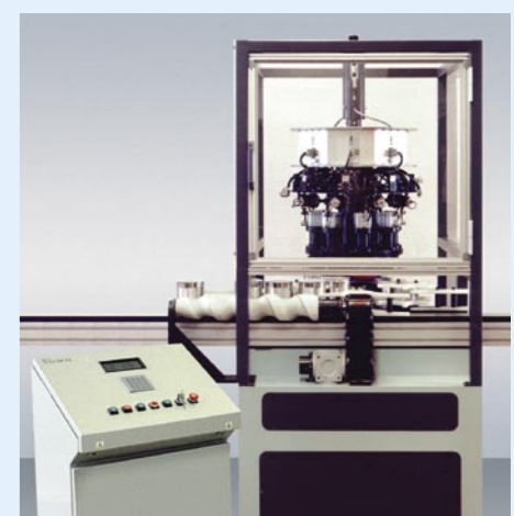
VPMS-2 clock-based system for 8 lines for inspection with high clock speeds
