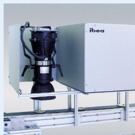
TIS image processing with heat flow thermography
