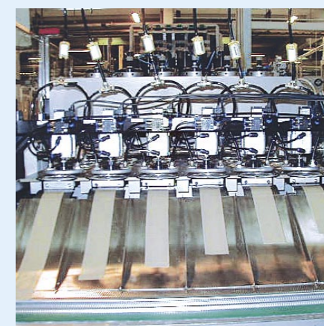
VPMS-1 cycled system for 6 lines for 99mm foil ends production
