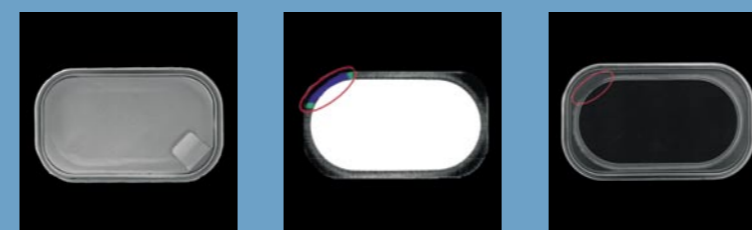
Non-destructive thermographic detection of faulty Easy-Peel-adhesions
