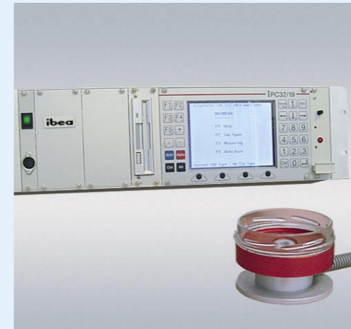
Flip-tester for inspection of closures and TO-caps
