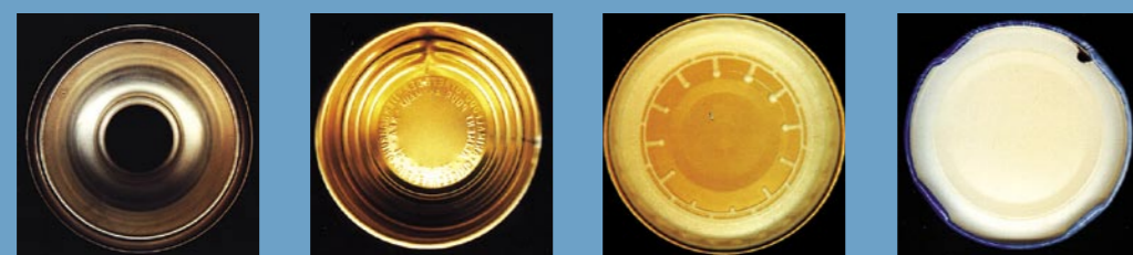
Detection of faulty objects via image processing for various end and can types
