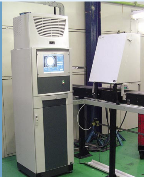
ViS-3 single lane inspection system for flat cans (Crown UK)
