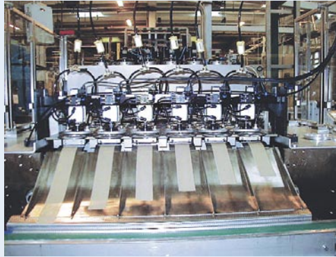
VPMS-1 Cycled system for 6 lines 99 mm easy peelable ends
