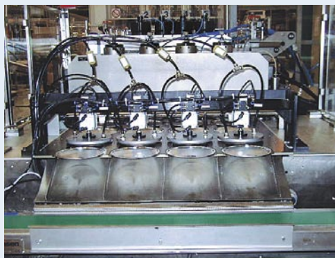
VPMS-1 Cycled system for 4 lines 153 mm easy peelable ends
