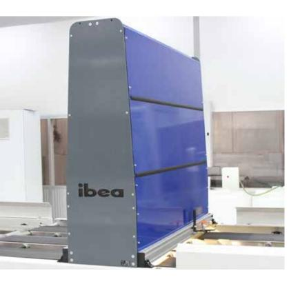
The BT Master SC scans the current processed production board and creates an image of all the located stones (bricks) and identifies its quality and location. Optionally, a 3D camera can be added to determine a height profile.
