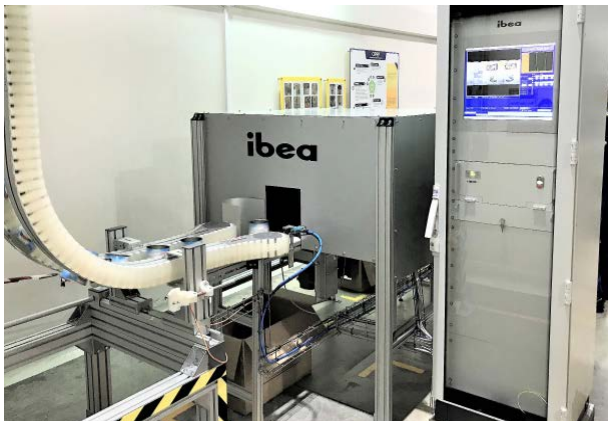
6 camera system with conveyor and computer rack
