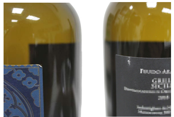
Defects at the label: Folded label and scratches in the design
