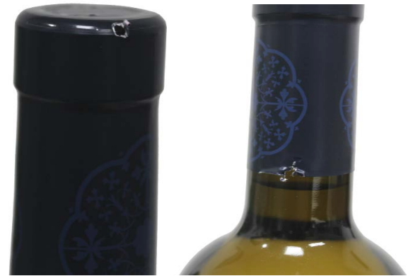
Defects at the bottle neck: Cracks at the lid and tear of capsule
